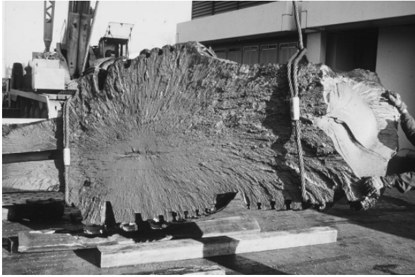
Fig. 10.1. Fatigue failure of a steam turbine shaft made of 28 NiCrMoV 85. The fragment shown has a mass of about 24 t. The crack started at a material defect within the shaft [3]
