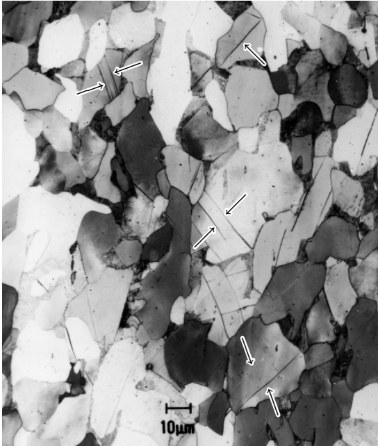
Fig. 6.56. Deformation twins in ferritic steel. The twinning planes can be observed as lines within the grains, some marked by arrows
